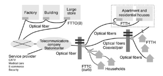
Fig. 2 Positioning of FTTH
